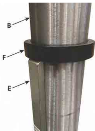
Figure 6-3: Remove Rack Ring and Rack
