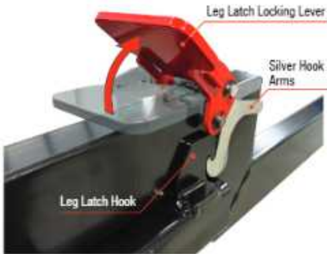
Figure 7-8: Unlocking Legs
