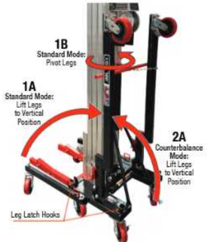
Figure 7-3: Positioning Legs to Vertical Position
