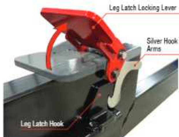
Figure 6-9: Unlocking Legs
