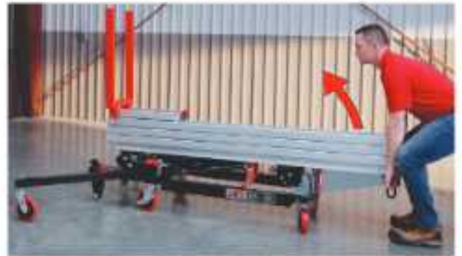
Figure 6-7: Lifting Mast to Vertical Position
