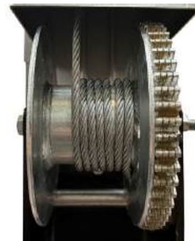
Figure 2-1: Cable Wrapped Tightly and Evenly
