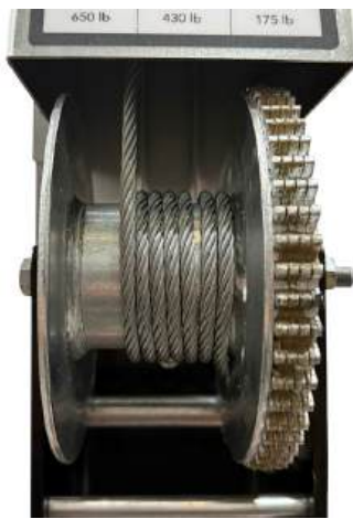
Figure 4-6: Cable Wrapped Tightly and Evenly
