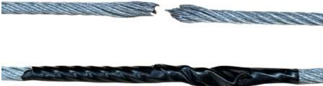
Figure 4-5: Spiral-Wrap Cable Ends
