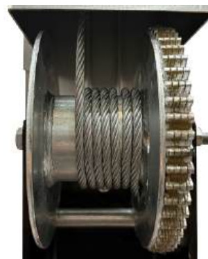
Figure 4-23: Cable Wrapped Tightly and Evenly
