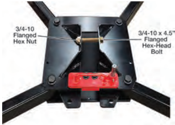
Figure 6-5: Removing Flanged Hex-Head Bolt and Nut
