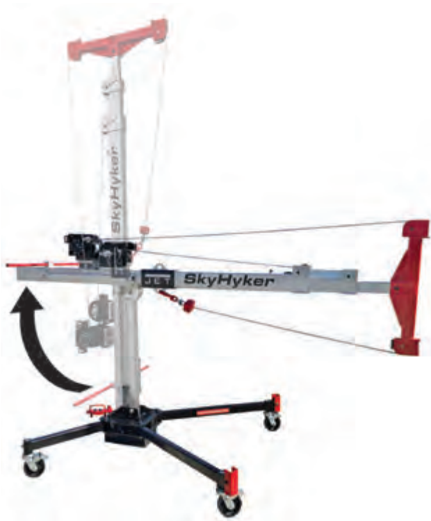
Figure 7-36: Rotating Mast to Travel Position
