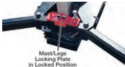
Figure 8-3: Mast/Legs Locking Plate in Locked Position
