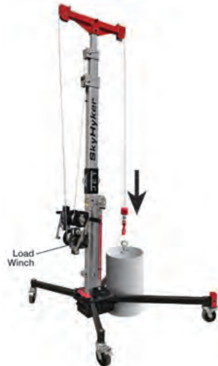
Figure 7-11: Lower Lift Cable to Object
