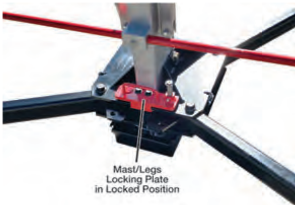
Figure 7-8: Mast/Legs Locking Plate in Locked Position
