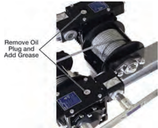
Figure 8-8: Adding Grease
