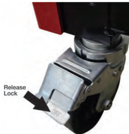
Figure 7-40: Engaging and Releasing Caster Locks
