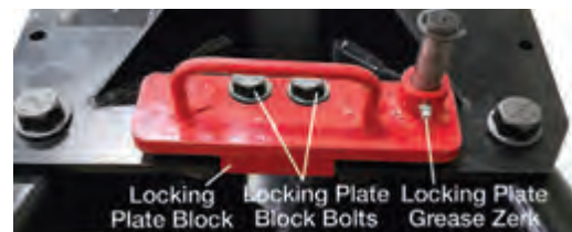
Figure 8-4: Mast/Legs Locking Plate Block and Grease Zerk
