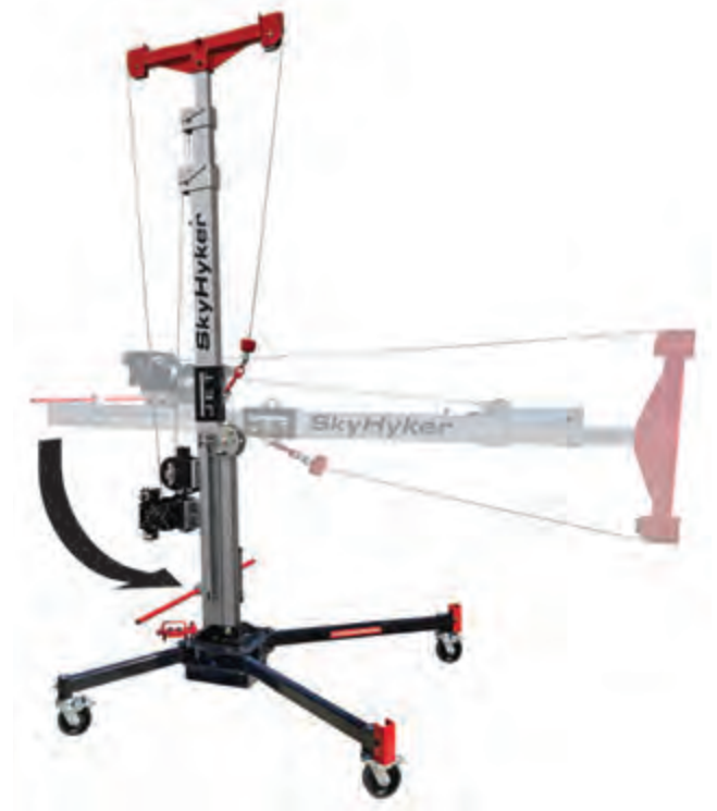
Figure 7-6: Rotate Mast to Load Position
