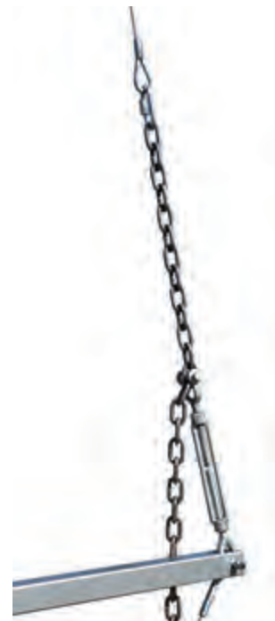
Figure 7-19: Hooking Chains to Turnbuckles
