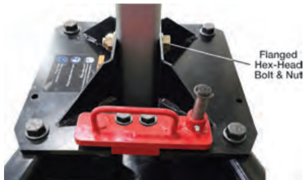
Figure 6-8: Attaching Square Tube to Base
