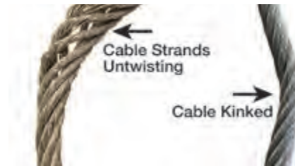
Figure 8-2: Cable Strands Untwisting and Cable Kinked
