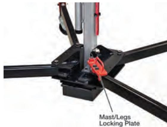
Figure 7-1: Mast/Legs Locking Plate Open
