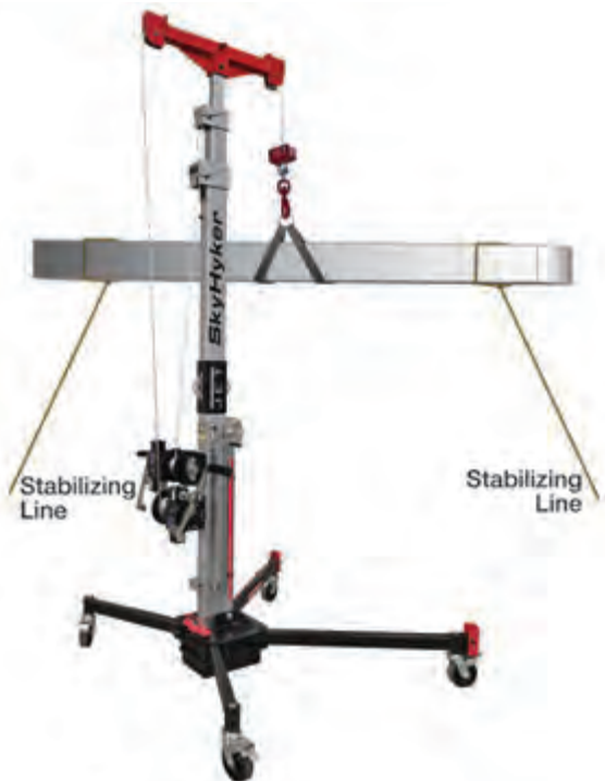
Figure 7-12: Using Stabilizing Lines
