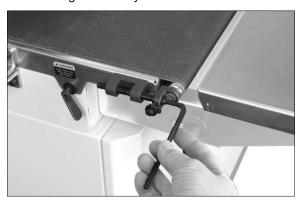
Figure 8-3: conveyor belt take-up screw
