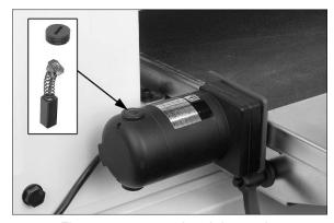
Figure 10-4: motor brush inspection
