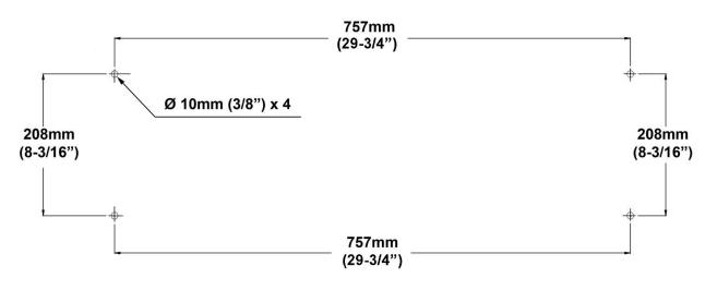
Figure 2 Clearance hole spacing for mounting lathe
