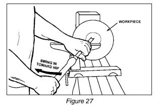
6. Use the left hand to control cutting edge of gouge, while right hand swings tool handle around toward your body (Figure 27). The flute should start out facing top of workpiece and rotate upward as it moves deeper into the bowl to maintain a clean even curve. As the tool goes deeper into the bowl, progressively work out toward the rim. It may be necessary to turn the tool support into the piece as you get deeper into the bowl.
