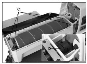
Figure 10-2: drum removal
