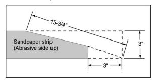
Figure 6-6: abrasive trimming – **JWDS-1632 ONLY** (not applicable to Ready-to-Wrap strips)
