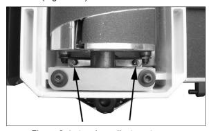
Figure 8-4: tension adjustment screws
