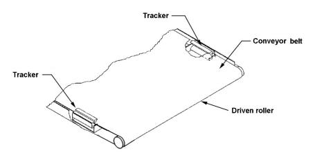
Figure 11-1: Underside of conveyor shown
