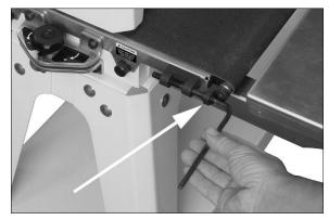
Figure 8-2: belt tension adjustment
