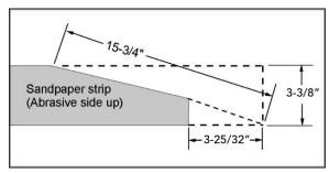
Figure 6-7: abrasive trimming - JWDS-1836 ONLY
