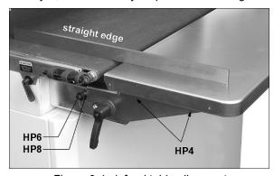
Figure 6-4: infeed table alignment
