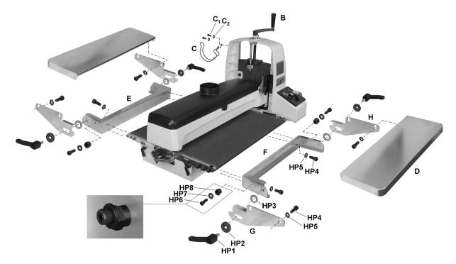
Figure 6-3: Assembly of Sander and OPTIONAL Infeed/Outfeed Tables
