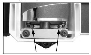
Figure 8-5: tension adjustment screws
