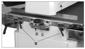
Figure 8-4: drum alignment
