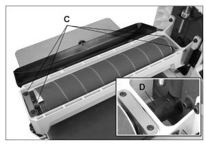
Figure 10-2: drum removal
