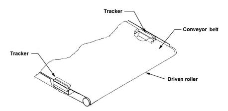
Figure 11-1: Underside of conveyor shown
