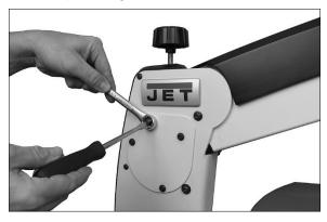
Figure 24: tightening arm lift
