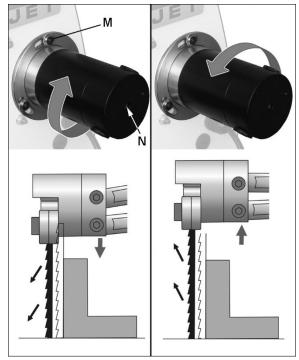
Figure 23: blade oscillation
