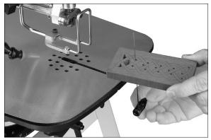
Figure 16: installing blade with workpiece
