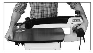
Figure 7: correct lifting
