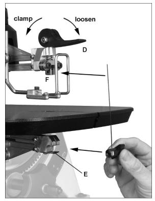
Figure 15: installing blade into guides
