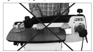
Figure 6: INCORRECT lifting
