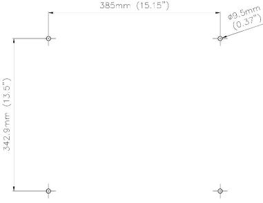
Figure 2: scroll saw mounting hole pattern
