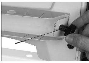
Figure 14: installing blade into holder
