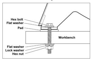
Figure 9: bench mounting (fasteners not included)
