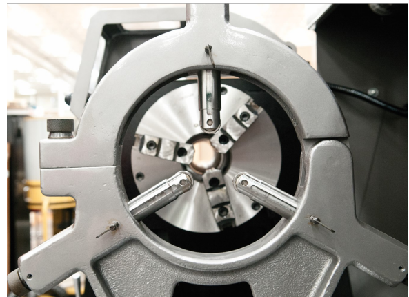
STEADY REST FEATURES DOUBLE SEALED BALL BEARING GUIDES FOR SMOOTH MATERIAL MOVEMENTS
